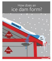
We have had significant snowfall this winter. Preventing ice dams, and heavy loads on roofs is important. An ice dam is an ice build-up on the eaves of sloped roofs of heated buildings that results from melting snow under a snow pack reaching the eave and freezing there. Freezing at the eave im-
